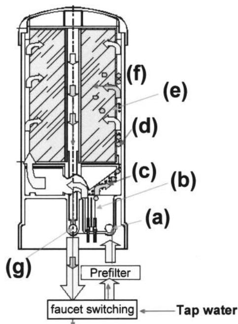
**Figure 1.** A structure of an NHE water production device. (a) Tap water inlet; (b) electrolysis tank equipped with three platinum-plating titanium electrodes; (c) electrolysis tank; (d) electrolytically produced hydrogen gas is collected; (e) high-pressure compressed activated carbon block; (f) the hydrogen gas that is dissolved in water is once stored up in a high-pressure compressed activated carbon block; (g) NHE water is taken out.
